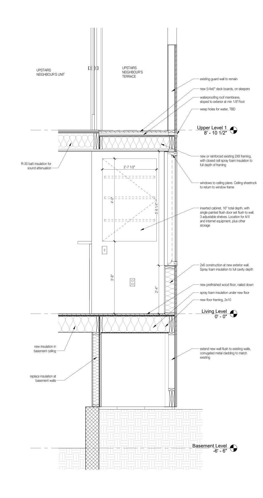
Detail Section at Floor Infill
